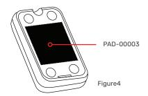
3 Remove the release liner from the back of another PAD-00003 and install it on the surface of the desired mounting location.
